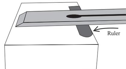
Note: By honing on and off the stone you avoid the risk of rounding the front edge of the blade which can occur if you stop short of the stone's edge. A slightly concave surface is better than a convex one.
