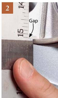
Measure the gap with a ruler calibrated to at least  $\frac{1}{32}$  in. or with a dial caliper.
