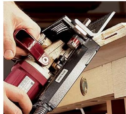
Cutting angle joints with a plate joiner is quick and easy. It's possible, but awkward, to do this with a router.
