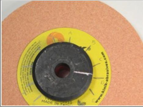
Now you can think logically of how you may begin to move and shim the washer to exert pressure to move the high spot of the wheel back towards the center line of the wheel. You could do this by random moves of the washer or applying shims, but the process goes quicker if you make some hash marks around the wheel's paper blotter label (NOT on the label underneath the outside washer or you will not be able to see them).
