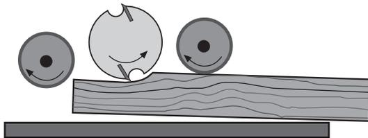
accounts for the phenomenon at least as well as the malevolence of the inanimate. If you do not fully support a board moving into or out of your planer, the free end drops, lifting the other end as it passes beneath the cutterhead. This lifting force is compounded by the action of the planer knives. As they sweep through a cut they contact wood only through the forward part of their
