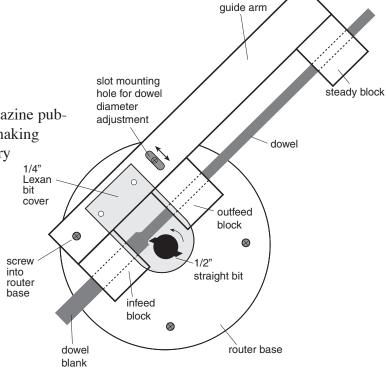
Make the guide arm and blocks blocks from 11/2" thick hardwood. Drill the outfeed and steady blocks to
