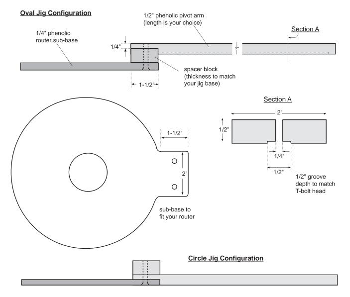
For routing circles, set the pivot arm flush with the sub-base as shown. Drill an 1/8" hole for a steel pivot pin (or simply drive a nail and clip it off 3/8" high) in the workpiece or in a piece of scrap attached to the work. Use a single T-bolt pivot, and adjust the cutting radius as needed.
