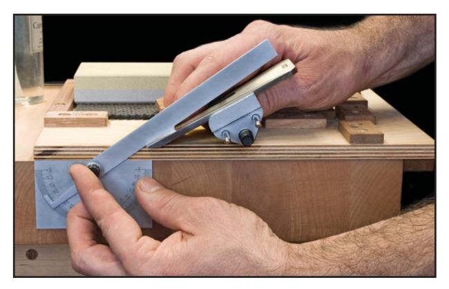
**Recommendations:** If you need additional or different angles, we suggest using a protractor to determine the projection distance. Hook your protractor under the edge of your jig, and place your blade (while in the honing guide) underneath the straight edge of the protractor. Adjust the position of the blade to match the angle of the protractor arm. The resulting projection distance gives you the position for the stop.
