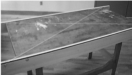
Adjust the rails until the two strings just kiss where they cross in the center of the bench. If you can't touch the upper
