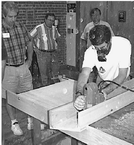
is typical of Tage's approach to woodworking: the concept is simple and the work itself quite straightforward. All you have to do is arrange for a router to move in a flat plane just above your workbench; set your depth of cut to skim the entire surface, and at the end of the exercise the benchtop will be flat. Nothing to it.
