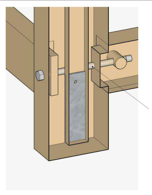
Bolt passes behind Crisscross mortise to engage barrel nut in front rail
