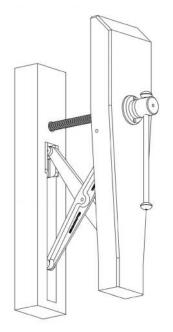
the other arm. With the pivot pin in place, set the chop/ leg upright and test the action of the Crisscross (you might want to clamp the leg to a bench to steady it.) The chop should now "float" in and out quite easily as the Crisscross supports the weight of the chop.
