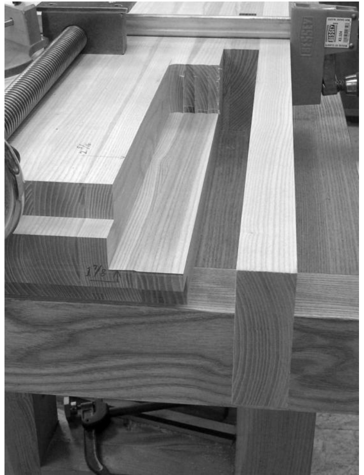
The completed cavity with dog strip and front laminate in place.
