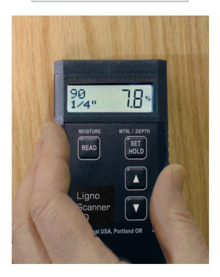
While measuring, you can toggle between the two measuring depths. Push the  $\blacktriangledown$  key to switch to 1/4" (20mm). Push the  $\blacktriangle$  key to switch to 3/4" (7mm). One hand can hold the meter, the other hand can activate the up or down key. You do not have to move the meter at all.
