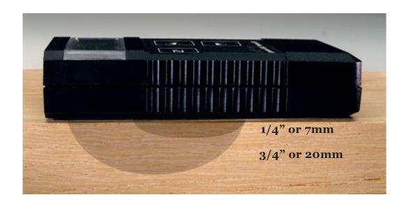
The measuring depth is crucial. For samples thinner than the measuring depth, readings may not be accurate:
