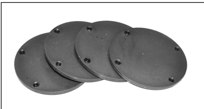
C10-392 ZERO CLEARANCE INSERTS - PK 4 Pack of four plastic inserts with table leveling screws. Inserts have no slot and require user to cut their own on installation. This minimizes the slot width so debris or thin cut wood strips will not catch or fall into the thin slot. Ideal for use when cutting small pieces on the bandsaw for inlay, shims, puzzles, etc.
