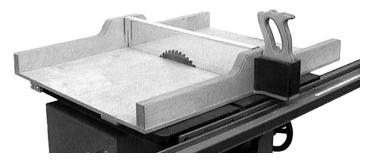
A SLIDING CROSSCUT TABLE is one of the most useful accessories you can add to your tablesaw. With good outfeed support and an accurate crosscutting system, your saw will be as safe, accurate and versatile as any in the business.
