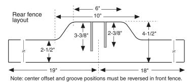
Each fence gets a couple of grooves milled into its inside face for mounting the clear plastic blade cover. One groove will be an inch longer than the other, and you'll shape the ends of the cover accordingly to give it two automatic height settings 1" and 2" above the table.
