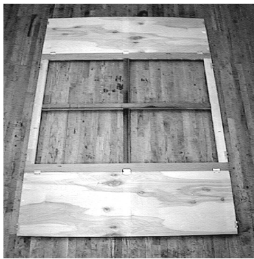
Figure 3 3/8" plywood folding top and bottom panels of are permanently attached to the filter frame with tight-pin hinges.
