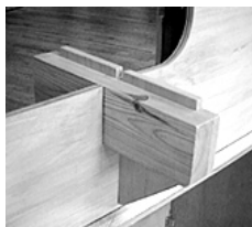
Figure 11 Simple brackets slip into notches in the back panel, making a platform to support a heavy duty fan.
