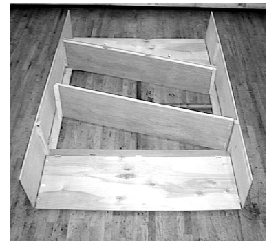
Figure 6 The side walls are folded up and horizontal panels are being deployed to form a large box behind the filter wall, from which air will be drawn through all four filters.
