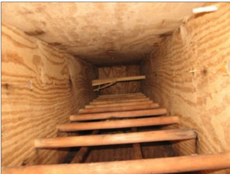
Inside view of the plywood steam box. Dowels create a support rack for your parts so steam will surround your work.
