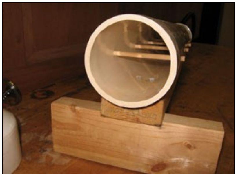
Inside view of PVC steam tube. 1/4" dowel rods support your work inside the tube and let the steam surround the wood.
