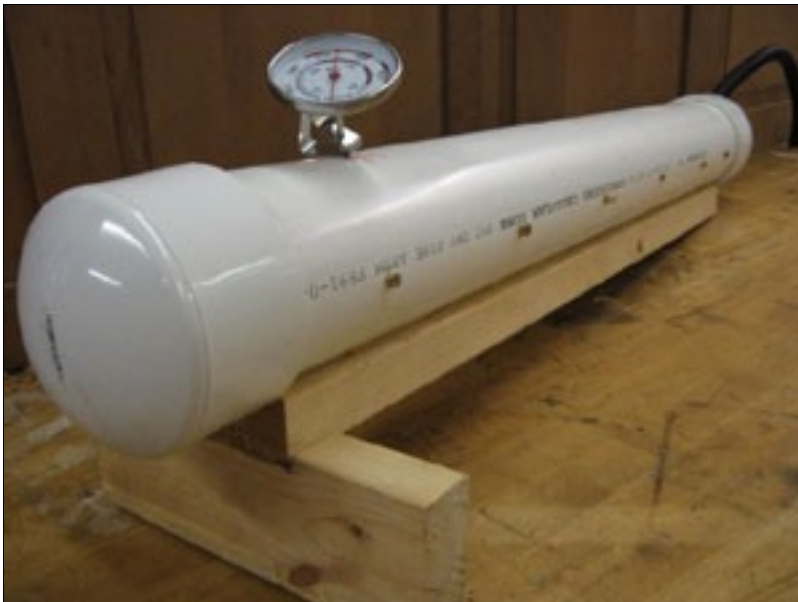
4" Schedule 40 PVC that is 36" long. (Shown with a meat thermometer inserted into a small hole at the top.)
