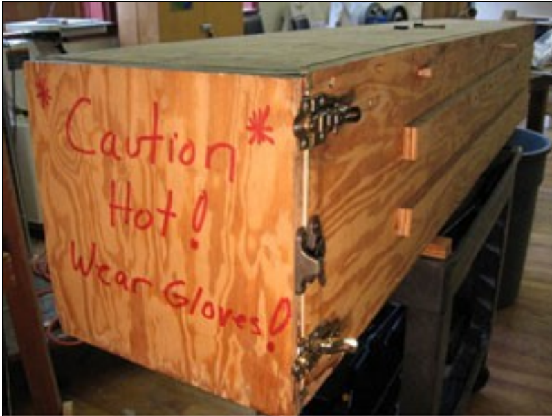
It's not pretty, but hey - it's a steam box. The center piece of hardware is a sash lock that draws the door tight to help seal the box.
