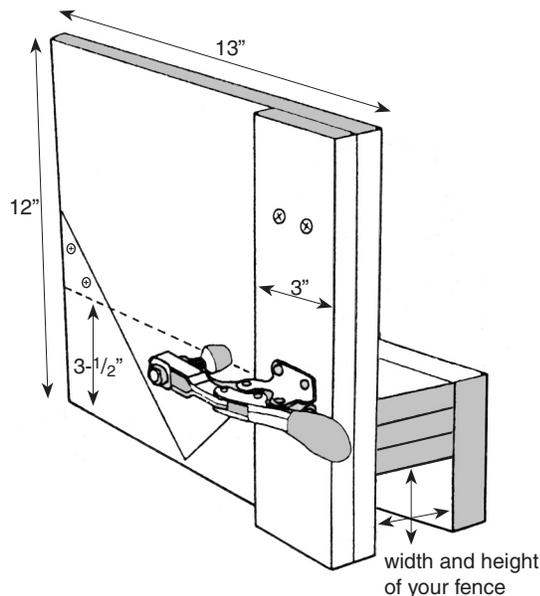
Now thickness plane or rip the piece to fit snugly between two pieces of stock clamped to your fence faces. The other dimensions shown in the drawing may be varied as needed to suit your work. I've used the jig on workpieces four feet long with no trouble controlling the stock. If you regularly need to cut tenons on large, long or heavy stock, consider adding another layer to the bridge and extra vertical pieces to widen the jig's footprint.
