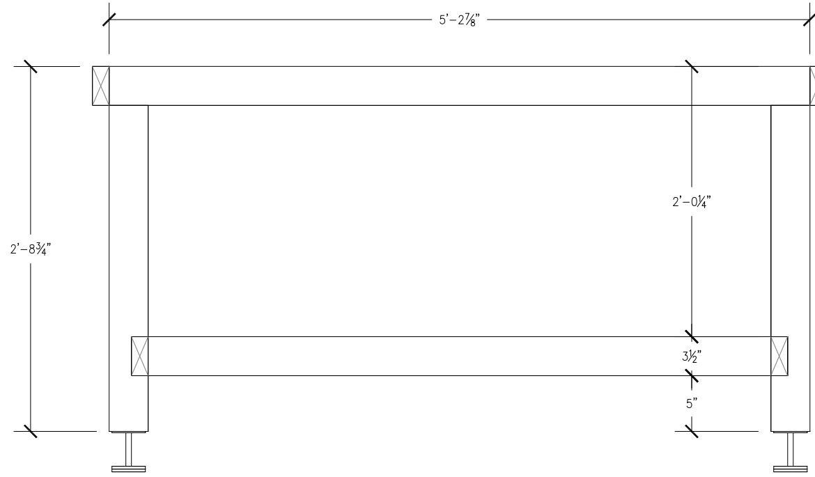
3 SIDE VIEW, LOWER FRAMING SCALE: 1" = 1'-0"
