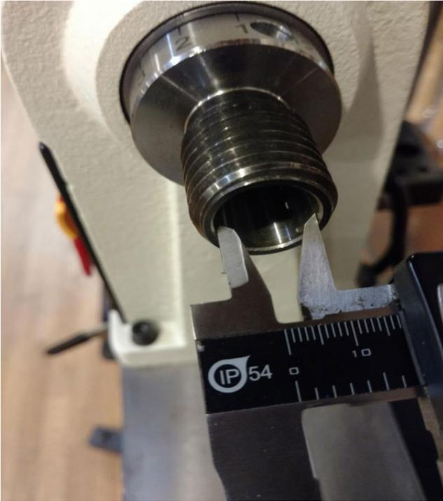
*Measure at the outer opening on the hollow socket of the headstock or tailstock.*
