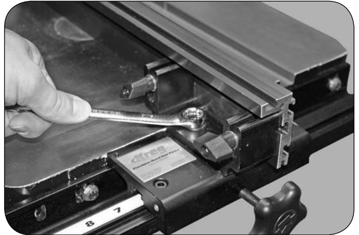
Loosen bolts on adapter bracket to pivot fence for blade drift.
