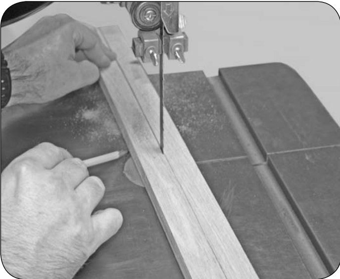
Scribe a line on the table surface of the band saw along either side of the scrap board.
