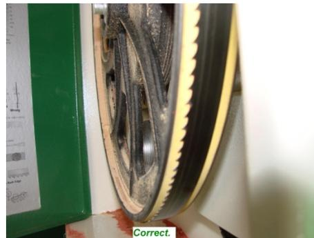
**If a blade is tracking on the rear of the lower wheel away from the door follow these steps:**
